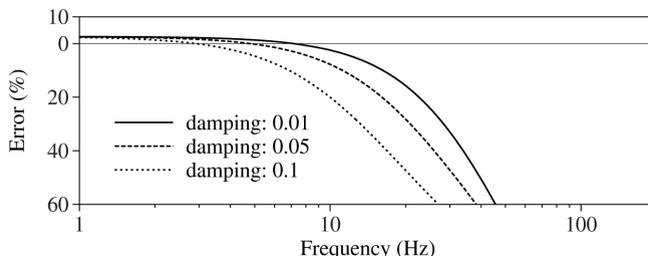
Fig. 6. Measurement error for the simple beam transducer with suspended mass of 5 kg for modal damping ratio values of 0.01, 0.05 and 0.1.
